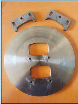
Extrusion Die for Soap Developed at TRTC, Guwahati
